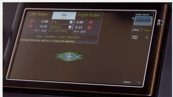
The screens user friendly interface projects a clear image of the rollers position and how they should be adjusted to the correct position.
